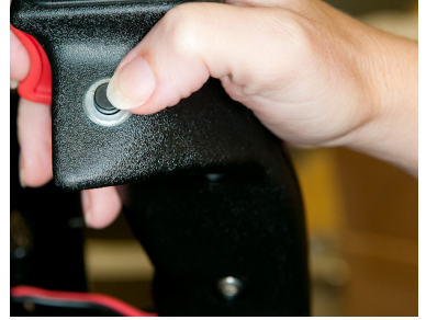
FIG 24 Only when both buttons are pressed will the unit engage and fire.
